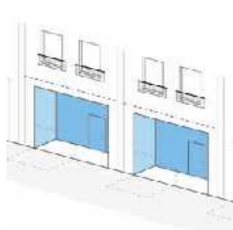
Figure 6.362 Illustrative example of a protected residential duplex entrance
