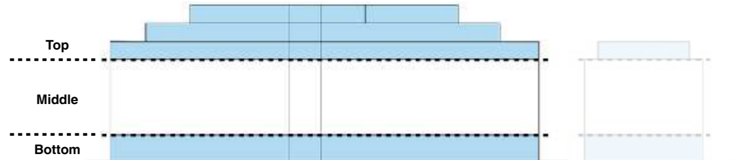
Figure 6.159 Plot C1A - North side reference elevation top, middle and bottom clearly defined by ground and roof treatments
