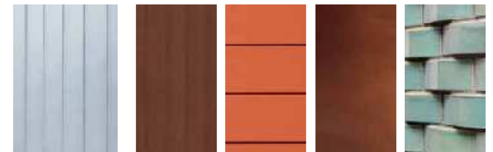
Figure 6.406 Acetylated or equivalent woods, terracotta, pre-oxidised and/or sealed/ coated pre-weathered metals and glazed brick/ tiles
