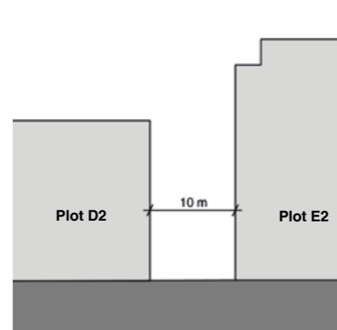
Figure 6.570 Building adjacency between D2 and E2
