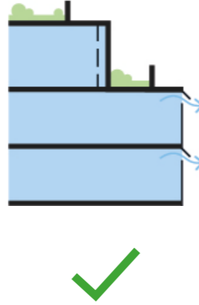
Figure 6.865 Option for operable/automatic sequenced openings to façade for natural/mechanically assisted natural ventilation
