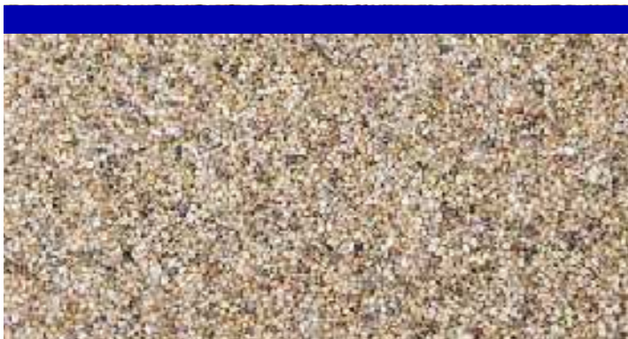
Figure 5.853 Resin bound gravel
