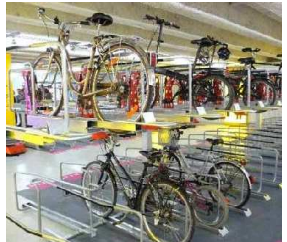
Figure 5.97 Two tier cycle storage system
