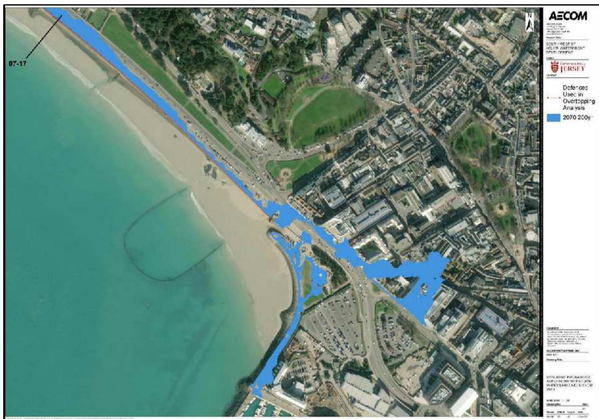
Figure 6-1: Areas of Overtopping Flooding for a 1:200SoP (2070) event (Existing Coastal Defence Structures)
