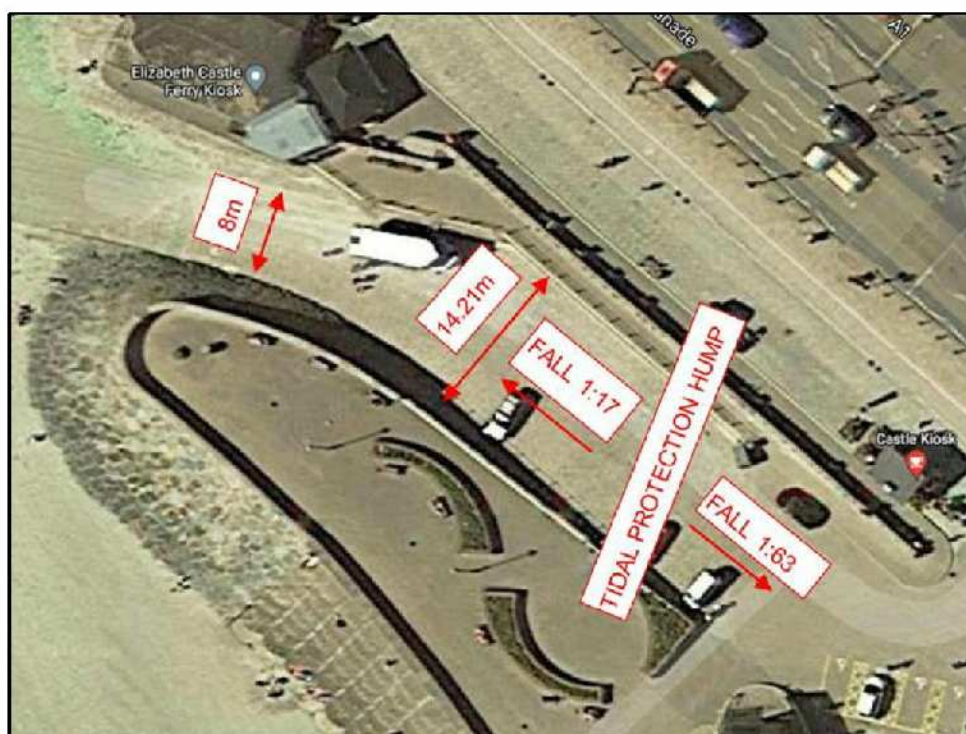
Figure 4-2 : Layout of existing slipway. Source: Google Earth, 2021
