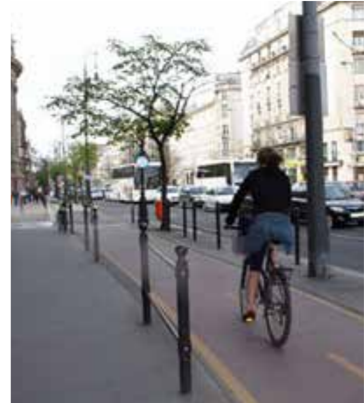
Figure 4.88 Bollards and kerbs should not be used to create separation between pedestrians, vehicles and cyclists
