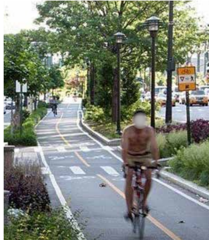
Figure 4.87 Planting must be used to create separation between pedestrians, vehicles and cyclists
