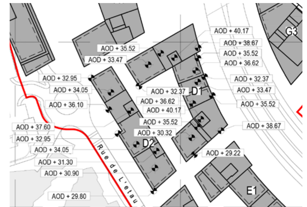
Figure 5.6 An example of maximum vertical parameters (Plot D) - Extract from drawing P12157-00-003-GIL-0014-01
