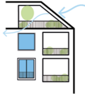
Figure 6.481 Inhabited pitch/mansard roofs for wind mitigation
