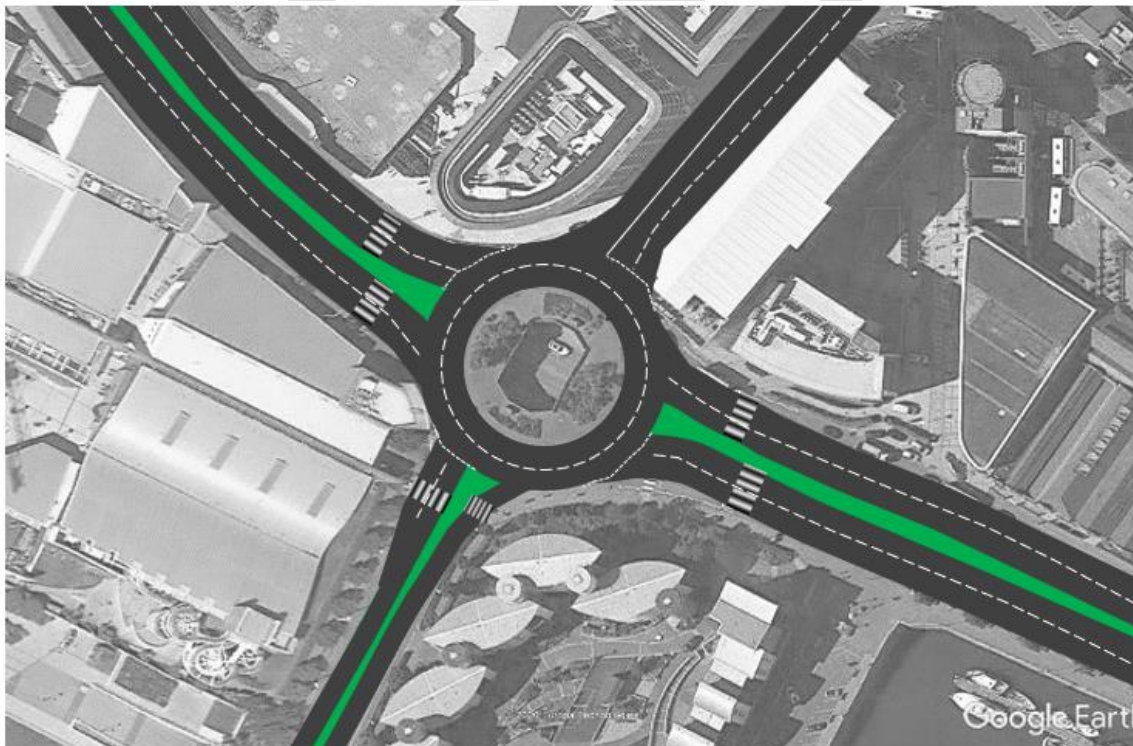
Figure 24 - Example of modified Castle St roundabout – two-lane approaches
